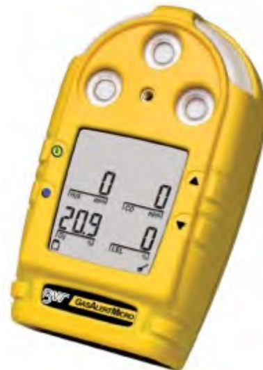
Photo 2-2. Typical Personal Four-Gas Monitor
