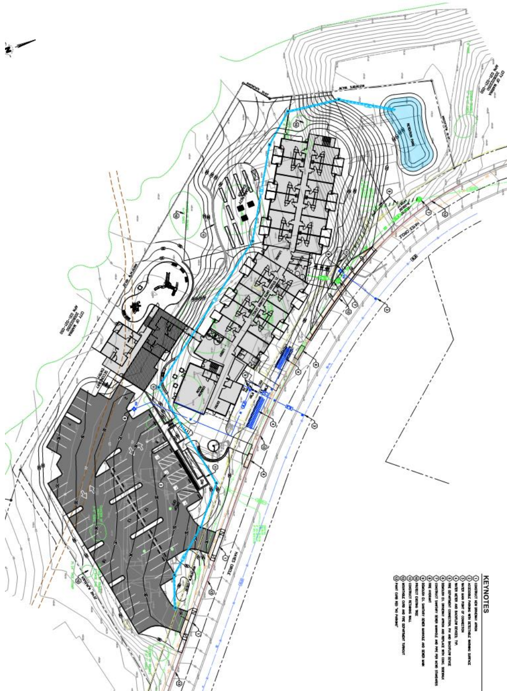
Site Plan showing the proposed Main Building (64 studios), Family Wing (7 two-bedroom units), and parking area (60 total spaces – 50 covered/10 uncovered)
